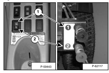
The lower left switch on the center console [Figure OI-44] controls the remote hydraulics when the selector valve is in the "A" position.
