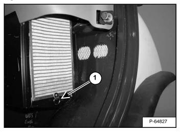
Remove the filter (Item 1) [Figure PM-13] and use a vacuum to clean the evaporator coils.
