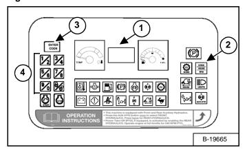
You can set the LCD (Item 1) [Figure SA-2] to show SPEED, HOURS, JOB clock or engine RPM.
