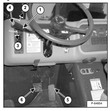
The Travel Direction Control Lever (Item 1) [Figure Ol-13] has three positions; Forward - PARK - Reverse (FPR).
