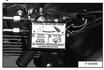
Move the selector lever to position "A" [Figure OI-43] for remote hydraulic operation.
