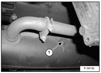
Remove the plug (Item 1) [Figure PM-43] from the cleanout hole in the muffler.
