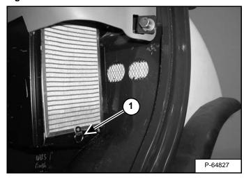
The recirculating filter is located on the right end of the heater / air conditioning housing.
