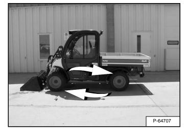
Rear tires usually wear faster than front tires. To keep tire wear even, move the front tires to the rear and rear tires to the front [Figure PM-46].
