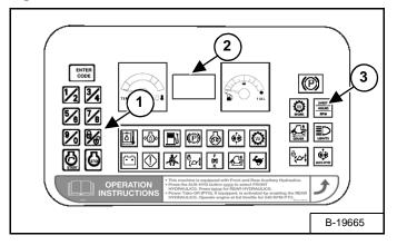
This allows the operator to Unlock the password feature so that a password does not need to be used every time you start the engine.
