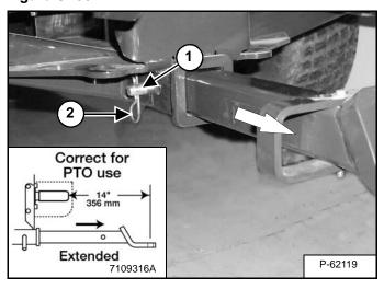
Extend the receiver hitch to the position shown (Inset) [Figure OI-30]. Install the receiver hitch pin in the hole (Item 1) and secure it with the retaining pin (Item 2) [Figure OI-30].
