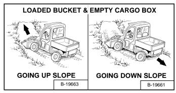
With a loaded bucket and empty cargo box, go up or down the slope with the heavy end toward the top of the slope [Figure OI-70].
