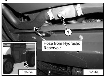
Remove the plug (Item 1) **[Figure PM-41]** from the fitting under the front end of the cargo box.
