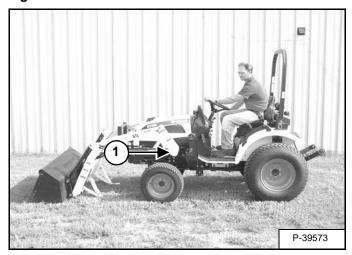
Remove the drain plug at the bottom of the differential (Item 1) [Figure PM-49].
