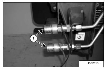
Remove the plugs from the quick couplers. Clean both the male and female couplers (Item 1) **[Figure OI-45]** before connecting.
