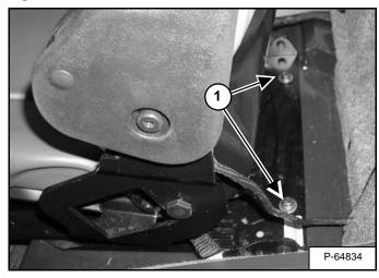
Remove two bolts (Item 1) [Figure PM-20] at the rear edge of the seat pan.
