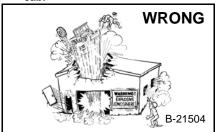
Do not use machine in atmosphere with explosive dust, explosive gas, or where exhaust can contact flammable material.
