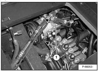
Loosen adjustment and mounting bolts (Item 1) [Figure PM-51].
