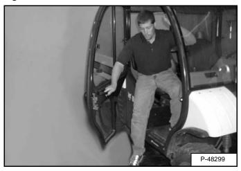
The cab door on the opposite side of the machine is used as an emergency exit [Figure OI-60].
