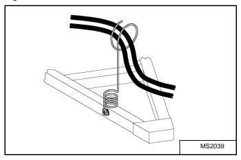
Secure the hoses to prevent damage [Figure OI-47].
