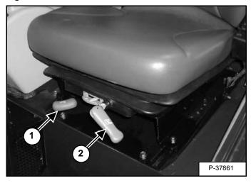
Release the lever (Item 1) [Figure OI-51] to adjust the seat distance from the steering wheel.
