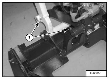
Each pivot pin is held in position with a bolt and lock nut (Item 1) [Figure PM-66].
