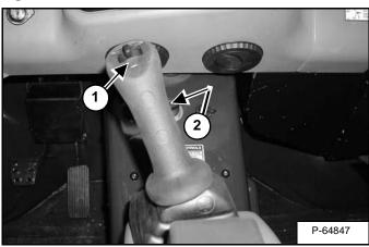
The switches on the joystick now control the rear auxiliary hydraulic functions (and PTO if equipped and connected).
