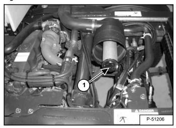
Remove the outer filter element (Item 1) [Figure PM-18] and, if required, remove the inner element (Item 1) [Figure PM-19].
