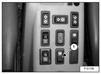
After auxiliary hydraulics is activated (Item 1) [Figure OI-21], press the high flow switch (Item 1) [Figure OI-22] on the center console. (The High Flow Icon on the switch will be ON.)
