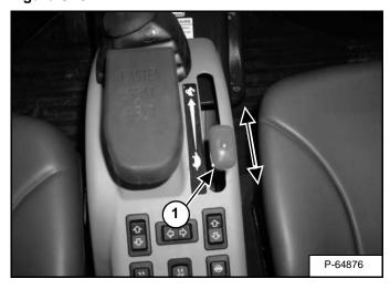
The engine speed control (Item 1) **[Figure OI-9]** is on the center console at the right side of the operator's seat. Move the engine speed control forward to increase the engine RPM and backward to decrease.
