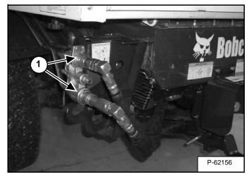
To connect the PTO motor, remove the hoses from the storage hooks. Connect the quick couplers (Item 1) [Figure Ol-28] to the rear auxiliary hydraulics by pressing the couplers together until they securely latch. (See REAR AUXILIARY HYDRAULICS (If Equipped) on Page OI-17.)
