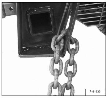
Fasten the rear of machine using the receiver hitch frame [Figure OI-83].
