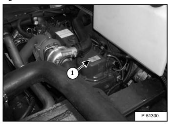
The engine serial number is located at the right end of the valve cover (Item 1) [Figure 2].
