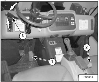
Gradually release pressure on the Drive Pedal (Item 1) [Figure Ol-14] until the machine comes to a complete stop.
