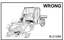
Disconnecting or loosening any hydraulic tubeline, hose, fitting, component or a part failure can cause lift arm or cargo box to drop. Do not go under lift arm or cargo box when raised unless supported by an approved lift arm or cargo box support device. Replace it if damaged.
