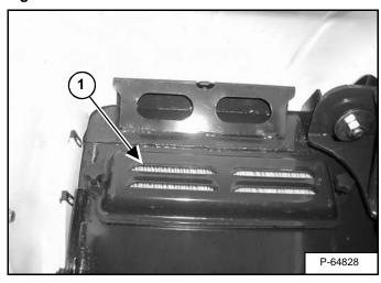
The fresh air filter is located under the right front fender [Figure PM-14].
