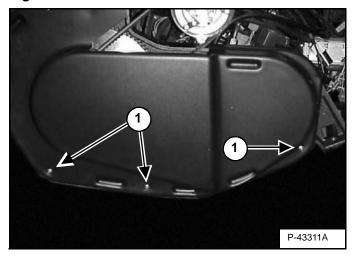
Remove the belt shield [Figure PM-52].
