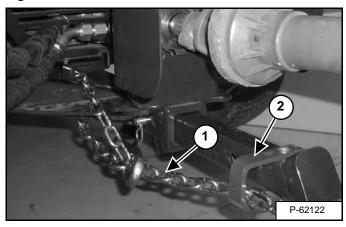
Route the safety chain (Item 1) [Figure OI-32] through the intermediate support (Item 2) [Figure OI-32] and fasten it around the hitch as shown. Allow no more slack in the chain than is necessary for turning.
