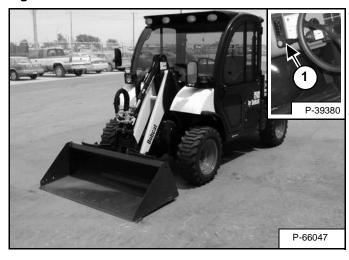
Lower the lift arm, put the attachment flat on the ground [Figure OI-58] and stop the engine.
