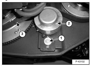
Loosen and remove the bolt (Item 1) [Figure PM-56] from the belt tensioner.
