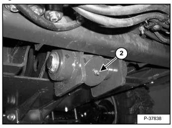
Base End Lift Cylinder (1) [Figure PM-58] (under machine).
