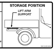
The Approved Lift Arm Support Device is stored under the cargo box on the passenger's side of the machine.
