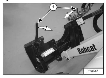
Move the Bob-Tach levers (Item 1) down to engage the wedges **[Figure PM-67]**. The levers and wedges must move freely.
