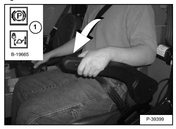
The TICS requires the operator to be seated in the operating position with the arm rest [Figure OI-7] fully lowered before the lift, tilt and traction functions can be operated. The seat belt must be fastened anytime you operate or are a passenger riding in the machine.
