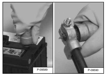
Always clean the battery terminals and cable ends when installing a new or used battery [Figure PM-36].
