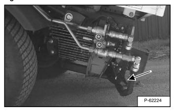
Remove the receiver hitch (if necessary) before loading or unloading to prevent it from hitting the ground [Figure OI-81].
