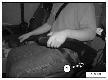
Use compressed air to clean any debris or dirt from the pivot parts (Item 1) **[Figure PM-2]**. Do not lubricate. Inspect all mounting hardware and tighten as necessary.
