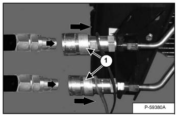
To Connect: Pull back on the collar of the female couplers (Item 1) [Figure OI-46]. Push couplers together, release the collar when the couplers are fully engaged and locked.
