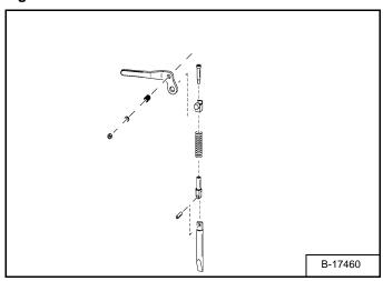
Inspect the mounting frame on the attachment and Bob-Tach, linkages and wedges for excessive wear or damage [Figure PM-69]. Replace any parts that are damaged, bent or missing. Look for cracked welds. Keep all fasteners tight. Contact your Bobcat dealer for repair or replacement parts.
