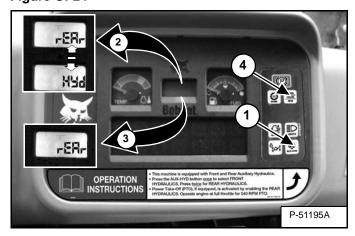
Press the auxiliary hydraulics button (Item 1) twice to activate the rear auxiliary hydraulics. The words **rEAr** then **Hyd** (Item 2) will flash several times on the display.
