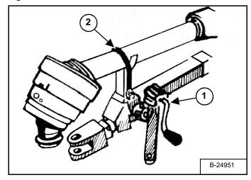
Use an approved jack to support the hitch of the attachment (Item 1) [Figure OI-40].
