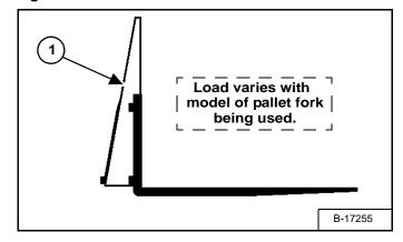
If a pallet fork attachment is used, the load center moves forward and reduces the load capacity.
