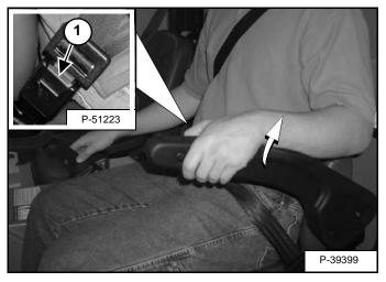
Press the red release button (Item 1) [Figure OI-59] to disconnect the seat belt.
