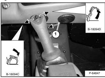
The thumb switch on the joystick now controls the front auxiliary hydraulic functions.
