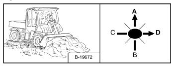
Lower the lift arm all the way (Item A) and tilt the bucket forward (Item D) **[Figure OI-72]** until the cutting edge is on the ground. Drive slowly forward to push the bucket slightly into the material.
