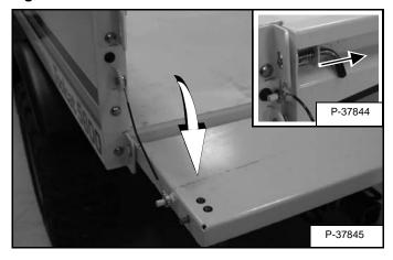
Release both latches and open the tailgate [Figure Ol-78].
