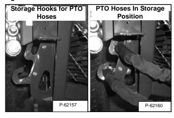
When the PTO motor quick couplers are disconnected, they can be stored in the hooks provided at the rear of the machine [Figure OI-27].
