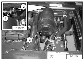
Replace the outer filter element only when the red ring (Item 1) **[Figure PM-17]** shows in the window of the condition indicator.
