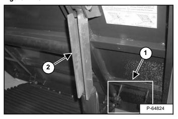
Remove the cargo box support device from the storage position (Item 1) [Figure PM-9].
