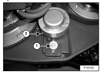
Loosen the bolt (Item 1) [Figure PM-53] on the spring loaded drive idler.
