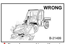
Never leave machine with engine running, with lift arm up, or with cargo box up.
