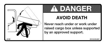
Raise the cargo box and install the approved lift arm support device.
