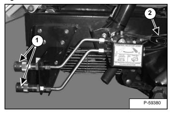
The quick couplers (Item 1) and the selector valve (Item 2) are mounted under the right side of the cargo box at the rear of the machine [Figure OI-42].
