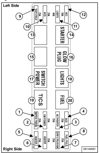
There is a decal **[Figure PM-35]** inside the fuse panel cover which shows location and size of fuses. Description and amp ratings (or relays) are also shown below.
