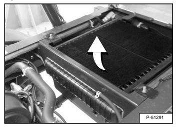
Lift up on the oil cooler to clean in between the oil cooler and the radiator [Figure PM-31].
