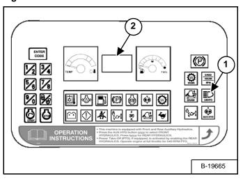
Turn the key on (Key Switch) or press ENTER CODE (Keyless). Press and hold the LIGHTS Button (Item 1) [Figure SA-1] for two seconds to view SERVICE CODES in the HOURMETER/CODE DISPLAY (Item 2) [Figure SA-1]. If more than one SERVICE CODE is present, the codes will scroll on the HOURMETER/CODE DISPLAY.
