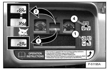
Press the Auxiliary Hydraulics button (Item 1) twice to activate the Rear Auxiliary Hydraulics/PTO. The words rEAr then Hyd (Item 2) will flash several times on the display. After a few seconds, the word rEAr (Item 3) [Figure OI-36] will remain on the display.
