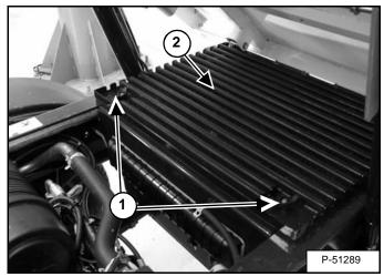
Remove the two debris screen wing nuts (Item 1) and remove the screen (Item 2) [Figure PM-30].
