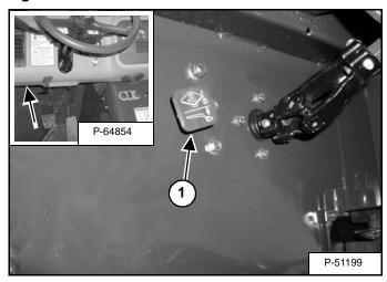
The lift arm by-pass is used to lower the lift arm in the event that you cannot lower the lift arm using the joystick.
