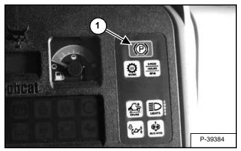
Press the button (Item 1) **[Figure OI-10]** to engage the parking brake. If the button is pressed, you must press it again to disengage.
