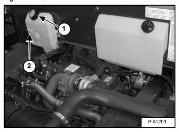
The coolant recovery tank (Item 1) [Figure PM-29] is located behind the cab.
