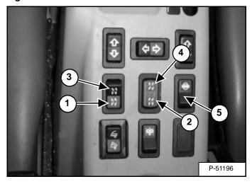
Put the Steering Mode Switch in All-Wheel-Steer (Item 1) [Figure OI-15].
