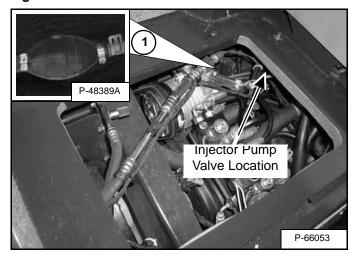
Open the valve (Item 1) [Figure PM-23] on the injector pump and squeeze the hand pump (Item 1) [Figure PM-24] several times until fuel comes from the valve with no air bubbles.
