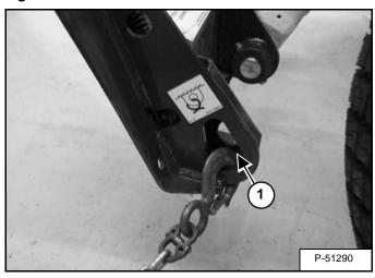
Fasten chains at the front using the tie down holes in the Bob-Tach (Item 1) [Figure OI-82].
