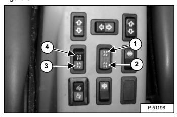
The steering mode can be selected either for Front Wheel Steer or All Wheel Steer operation.
