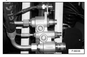
Front auxiliary hydraulics [Figure OI-18] are standard.
