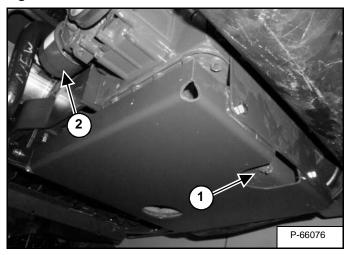
The engine oil drain and filter are located under the machine at the front end of the cargo box.
