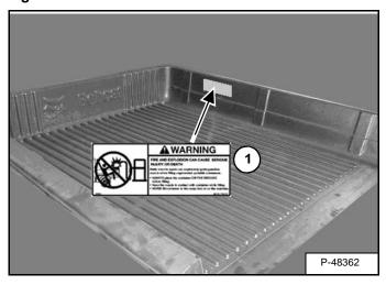
Cargo Box Liner (Option) has a Warning decal (Item 1) [Figure PM-25]. Replace if damaged or missing.
