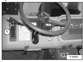
To check the function of the Neutral Start System, place the Travel Direction Control Lever (Item 1) [Figure PM-5] in FORWARD and turn the key switch to START position. The engine must not start.
