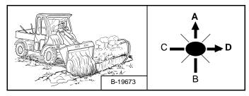
Lower the lift arm (Item A) [Figure OI-76] and put the cutting edge of the bucket on the ground (Item D) [Figure OI-76]. Drive forward to the edge of the hole to push the material into the hole.
