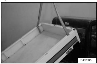
Install lift straps (or chains) through the stake holes at the front of the cargo box [Figure PM-10].
