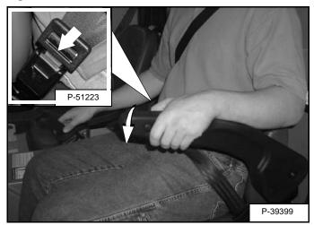
Fasten the seat belt snugly and lower the operator arm rest [Figure OI-53]. Adjust the belt so that it fits snug around the lower part of your hips. Passenger must also fasten seat belt.
