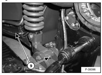
Lower Link (Front and Rear end of Link - Both Sides)
