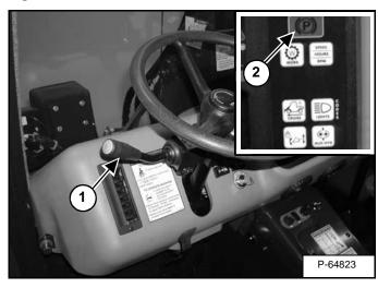
When the Travel Direction Control Lever (Item 1) [Figure PM-11] is in PARK, the Parking Brake is engaged.
