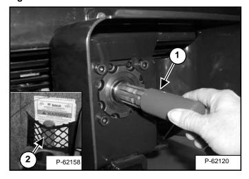
Remove the plastic PTO shaft sleeve (Item 1) [Figure Ol-33]. Keep the sleeve for use later when no PTO driveline is attached. It keeps dirt and debris off the shaft splines. Store the sleeve in the Handbook pouch (Item 2) [Figure OI-33] in the cab of the machine.
