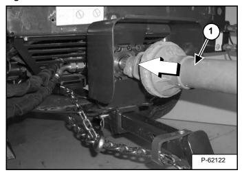
Connect the PTO driveline (Item 1) [Figure OI-34] to the PTO motor shaft. Make sure it is securely connected.
