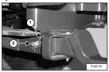
Remove the retaining pin (Item 1) [Figure OI-29] and then remove the receiver hitch pin (Item 2) [Figure OI-29].
