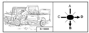
While raising the lift arm (Item B), tilt the bucket forward (Item D) **[Figure OI-74]** to keep it level and help prevent material from falling off the back of the bucket.
