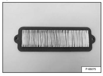
Remove the filter and shake it or use low air pressure to remove dirt **[Figure PM-15]**. The filter can be cleaned several times in this manner then it must be replaced.
