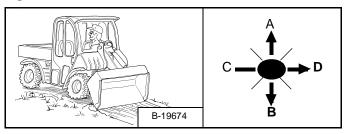
Raise the lift arm (Item B) and tilt the bucket forward (Item D) [Figure OI-75].
