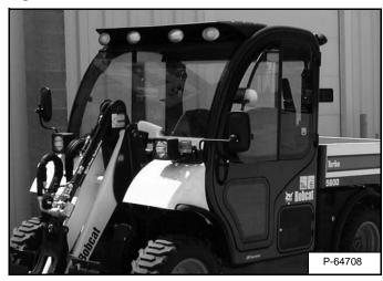
The machine has an operator cab (ROPS and FOPS) [Figure PM-12] as standard equipment to protect the operator from rollover and falling objects. The seat belt must be worn for rollover protection. Check with your dealer if the operator cab has been damaged or modified.
