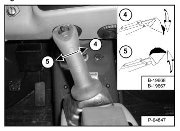
Movement of the joystick [Figure Ol-16] and [Figure Ol-17] controls the hydraulic cylinders for the lift and tilt functions.
