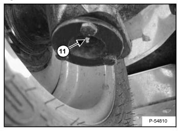
11. Front Bearing Pivots (Both Sides) (2) [Figure PM-64].
