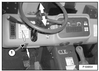
Release the steering column lock (Item 1) [Figure OI-52] and move steering wheel up or down for comfortable operation. Push lock up to secure.
