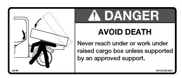
Raise the cargo box and install the approved cargo box support device. (See CARGO BOX SUPPORT DEVICE on Page PM-13.)
