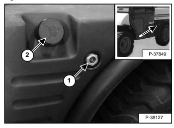
Check the fluid level in the sight gauge (Item 1) [Figure PM-39]. The fluid level is correct when at the center of the sight gauge.
