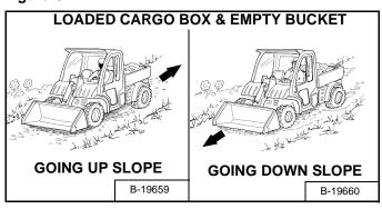
With empty bucket and a loaded cargo box, go down or up the slope with the heavy end toward the top of the slope [Figure OI-71].
