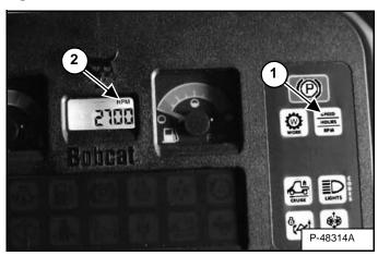
To Set 2700 RPM Engine Speed: Press SPEED/HOURS/RPM button (Item 1) [Figure OI-39] until RPM appears in display (Item 2) [Figure OI-39].
