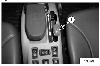
Push the engine speed lever (Item 1) **[Figure OI-38]** forward to increase engine speed to 2700 RPM (+/- 10 RPM). The engine must be operated at 2700 RPM for 540 RPM PTO operation.
