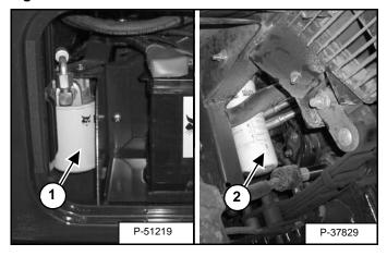
Remove the case drain filter (Item 1) [Figure PM-40].
