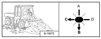
Raise the lift arm (Item B) and tilt the bucket backward (Item C) [Figure OI-73].
