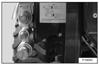
The quick couplers are located under the left side of the cargo box near the rear of the machine [Figure Ol-23].
