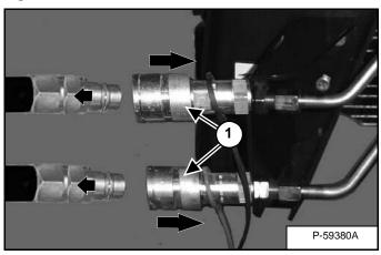
To Disconnect: Pull back on the collar (Item 1) [Figure OI-48] and pull the male coupler out to disconnect.
