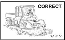
Never use machine without operator cab with ROPS and FOPS approval. Always fasten your seat belt.
