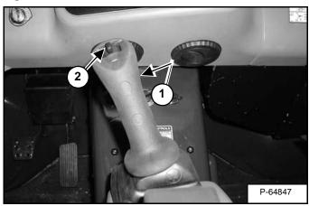
The trigger switch (Item 1) [Figure OI-26] on the front of the joystick can be used for continuous flow. Move the thumb switch (Item 2) [Figure OI-26] to the desired direction, then press and release the trigger switch. Release the thumb switch.
