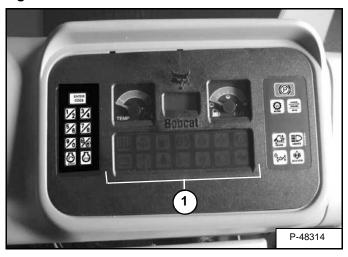
After the engine is running, frequently monitor the display controller panel [Figure OI-57] for error conditions.
