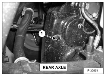
Remove the check plug (Item 1) [Figure PM-47] & [Figure PM-48] from the front or rear housing.
