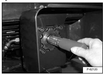
Put the plastic sleeve on the PTO shaft [Figure OI-41] to prevent dirt and debris from collecting on the PTO shaft splines.
