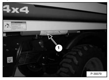
Remove the lift arm support device (Item 1) [Figure PM-6] from the storage position under the right side of the Cargo Box.
