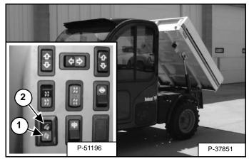
Press the back of the switch (Item 1) **[Figure OI-79]** to raise the cargo box. Press the front of the switch (Item 2) **[Figure OI-79]** to lower.
