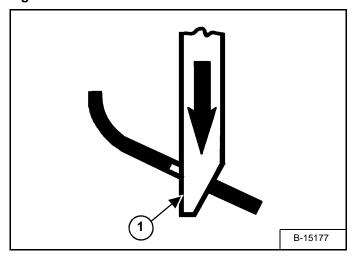
The wedges (Item 1) **[Figure OI-67]** must extend through the holes in the mounting frame of the bucket (or attachment), securely fastening the bucket or attachment to the Bob-Tach.
