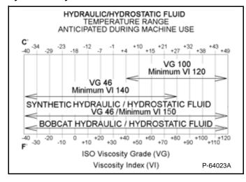
If needed, remove the fill cap (Item 2) [Figure PM-39] and add fluid. (See chart above.)
