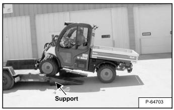
A machine with an attachment must be loaded or unloaded forward. A machine without an attachment can be loaded or unloaded either forward or backward [Figure OI-80].
