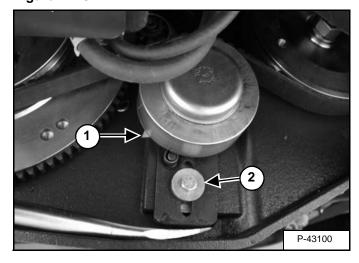
Use a pry bar to push the idler assembly against the belt, the pointer (Item 1) **[Figure PM-54]** will be at the 9 o'clock position when the idler stop is bottomed out.
