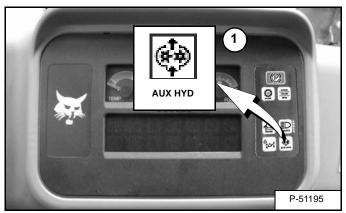
Press the auxiliary hydraulics button (Item 1) [Figure Ol-19] to activate the front auxiliary hydraulics.
