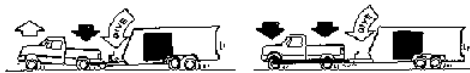
(LEFT) Trailer "Dive" during heavy braking increases the effect of tongue weight. (RIGHT) Weight distributing hitch transfers loads to frame and to both axles of tow vehicle for safer stops and smoother ride.
