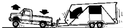
Top heavy loads can cause trailer "dive" under hard braking, possibly reducing steering and braking control.
